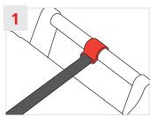
Position rear clip over lid hinge at desired location and snap-on
